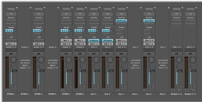
This DTDM Mixer example features six audio channel strips, two aux channel strips, two instrument channel strips, and two stereo sums. The eight output signals of the DTDM Mixer example shown above are routed into the TDM Mixer. The DTDM Mixer output signals are received by the ESB TDM inputs—chosen as TDM aux channel strip input sources.
